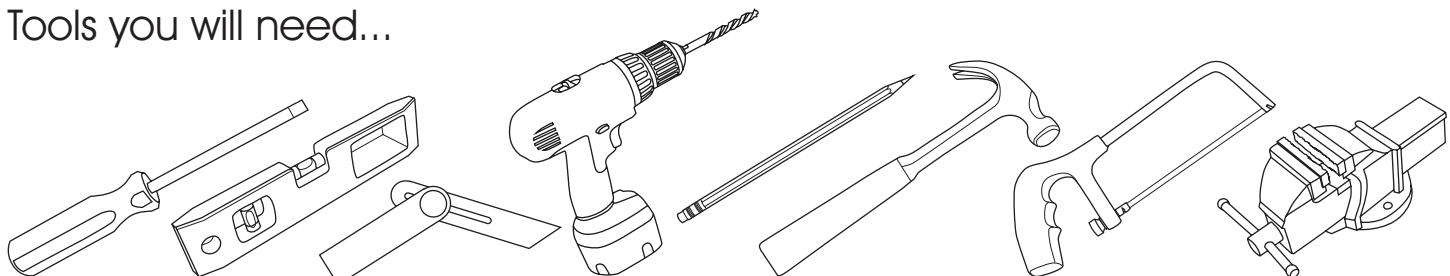
Flathead Screwdriver      Spirit Level      Bevel or Protractor      Drill      Pencil      Hammer\*      Hacksaw\*      Vice\*
